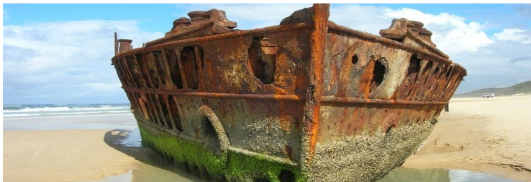
Graph I: Corrosion attack on an old ship
